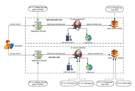
Figure 2: Secure & non-secure CDP with incorporated security tactics.
